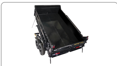
All GT models come standard with a 10ga. steel bed.
