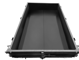
Easy to clean 10-12ga steel bed and sidewalls
