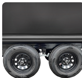
The deck over features no fenders allowing a wider bed area.
